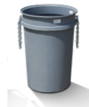
Chute Section TRS-CH Overall Ht. 48" Max. Usable Ht. 42" Top Diameter 32" Bottom Diameter 28"
