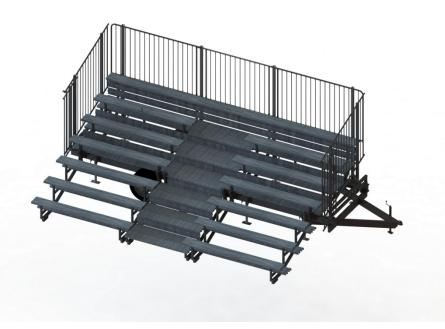
Step 4) Unpin mid-aisle handrails from their storage position on the back of the bleacher. Install both of these in the center of the aisle, in the pre-attached handrail mounting brackets, and reinstall the snap pins (2 per handrail) in the hole underneath the bleacher boards.
