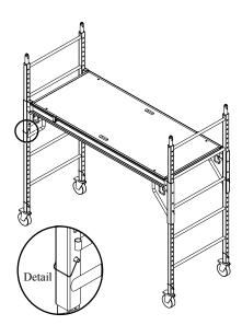
5) For additional security insert 2" snap pins through the "U" channel and frames after the platform height has been properly set.
