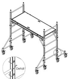
7) Attach the remaining three outriggers as described in step 7. Make sure that the casters on the outriggers are level with the casters on the ladder frames.
