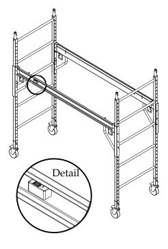
4) (A)Then lay a plywood platform on the braces. Line up the 4 holes in the plywood with the pins on the arm braces. (B)Turn the platform hold down devices so that they "trap" the platform onto the braces.
