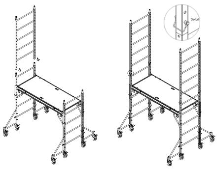
9) Attach the second level arm braces, one at a time, as described in **Step 2** and position them to the desired location on the second level ladder frames.
