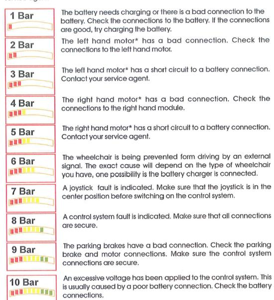
\* If the programmable parameter, Motor Swap has been enabled, then left and right hand references in this table will need transposing.
