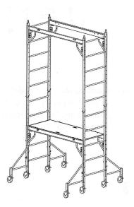
9) Attach the second level arm braces one at a time as described in step 2 and position them to the top of the second level ladder frames.
