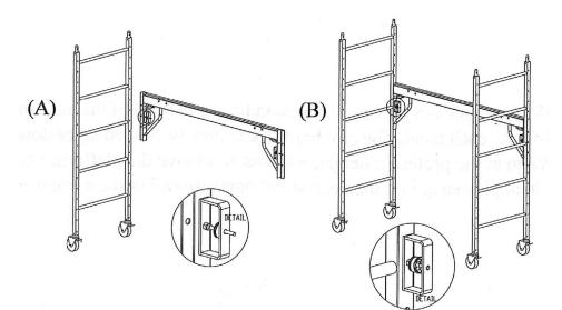
2) (A)Turn the frames right side up and engage the lock on the casters. While holding one end frame with one hand use your other hand to pull back the lock pin on the arm brace and engage the "U" channel over the frame leg.
