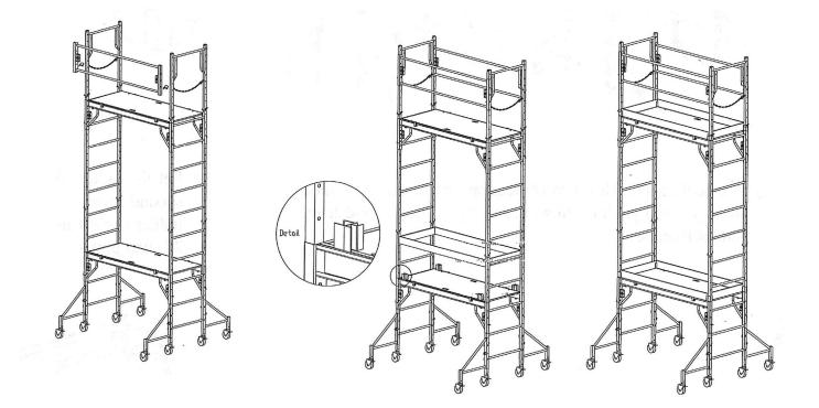
12) Attach the guard rail side panels using the same procedure (step 2)used to attach the arm braces. After their height has been set, secure them with 2" snap pins.
