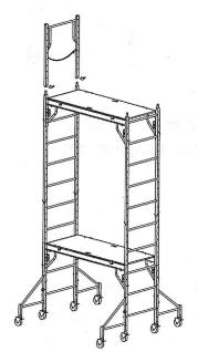
11) Lay a plywood platform on the braces. Then line up the four holes in the plywood with the pins on the arm braces. Turn the platform hold down devices so they "trap" the platform onto the braces. Then secure the braces using 2" snap pins through the "U" channel and the frames.
