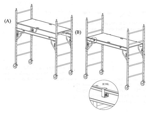
3) Attach the second arm4)brace as described in step 2.plyMake sure both arm braces aredepositioned at the same level.TheBe sure the platform hold downThedevices are turned out of thetheway.ca
