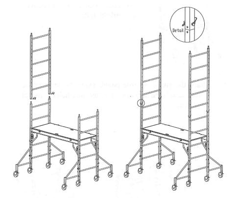
8) Set the ladder frames for the second level on the first level ladder frames and secure with 2" snap pins.
