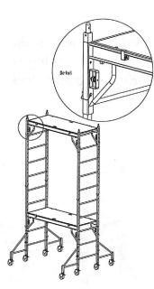
10) Lay a plywood platform on the braces. Then line up the four holes in the plywood with the pins on the arm braces. Turn the platform hold down devices so they "trap" the platform onto the braces. Then secure the braces using 2" snap pins through the "U" channel and the frames.
