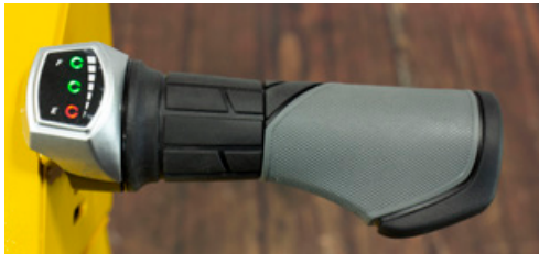
Battery indicator light and twist throttle.
