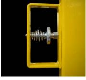
User friendly squeeze-lock is spring loaded to maintain the locked position at all times except when released for adjustment. A locking knurled knob is provided to prevent unintentional release. Additional snap pin is provided as a dual locked scaffold system.
